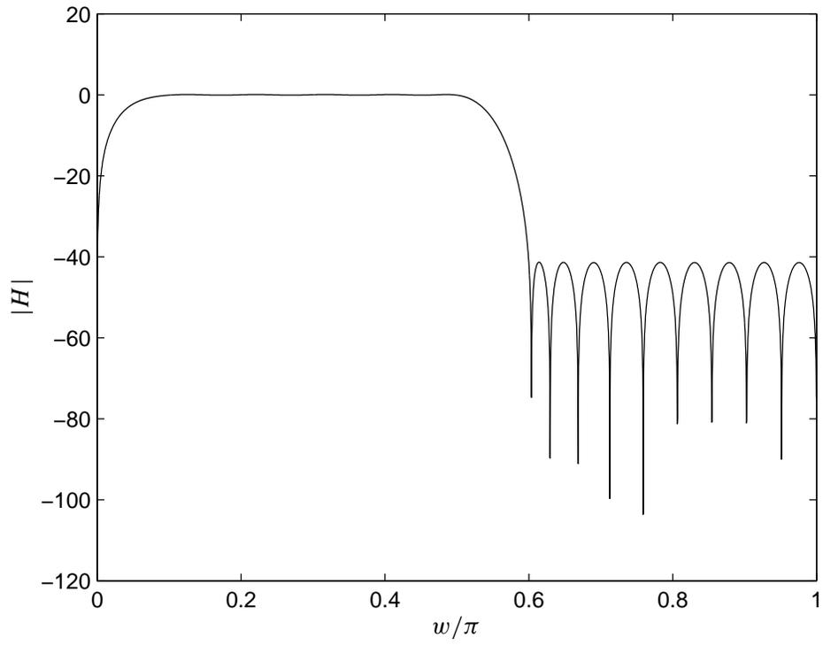
Figure 21: The magnitude of the frequency response of the filter
