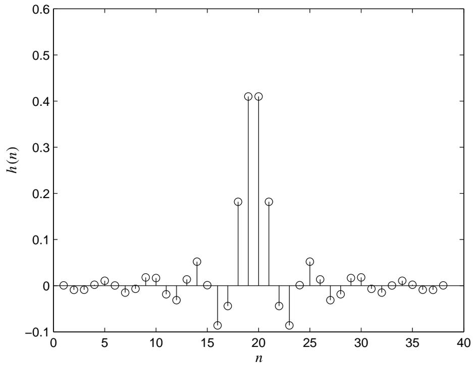
Figure 17: Impulse response coefficients of the FIR filter
