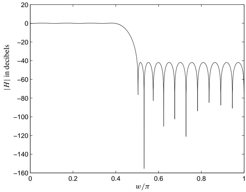
Figure 18: Magnitude of the frequency response of the FIR filter
