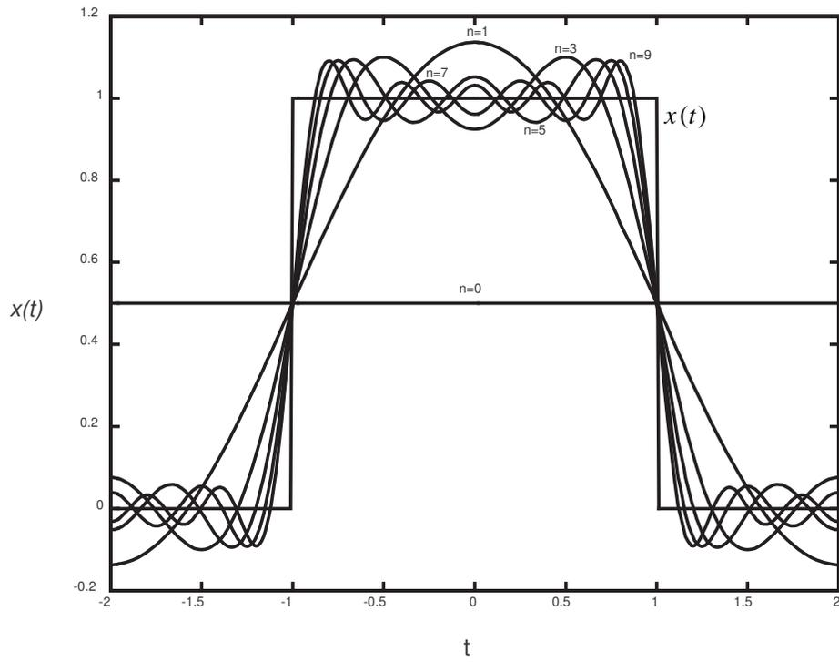
Figure 1: Various Fourier series approximations for the rectangular pulse in Computer Problem 1
