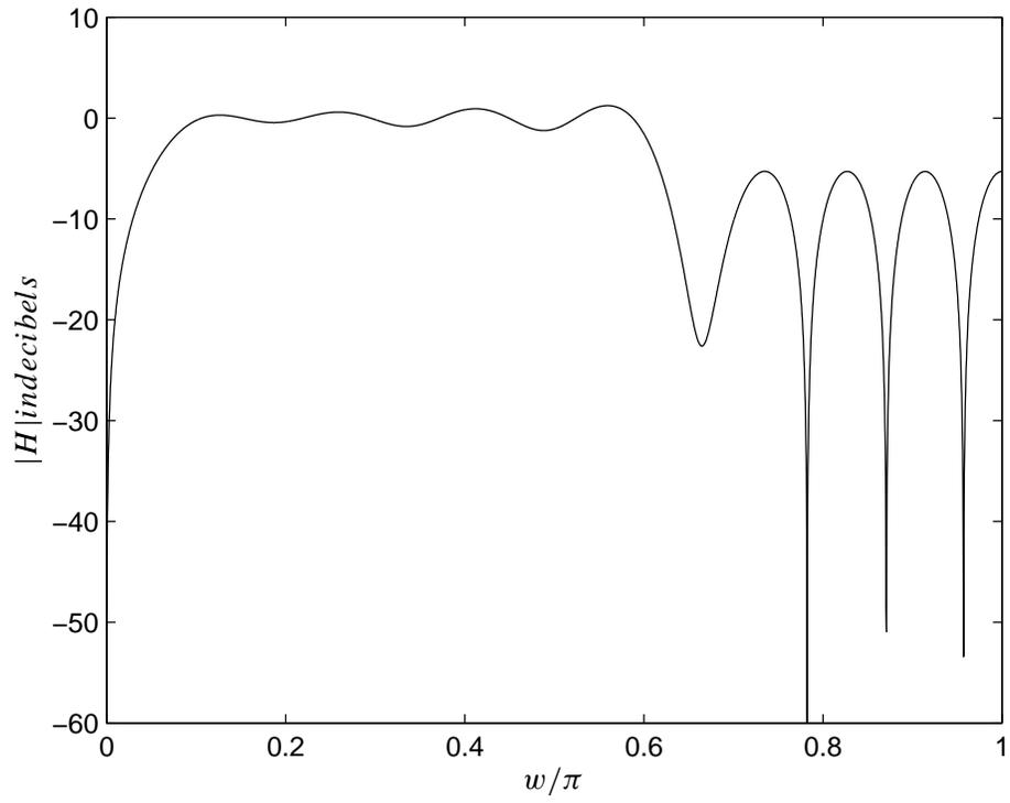
Figure 23: Magnitude of the frequency response of the filter
