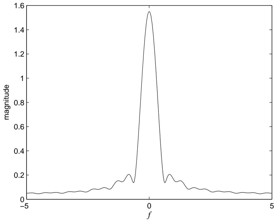
Figure 5: The common magnitude spectrum of the signals  $x_1(t)$  and  $x_2(t)$
