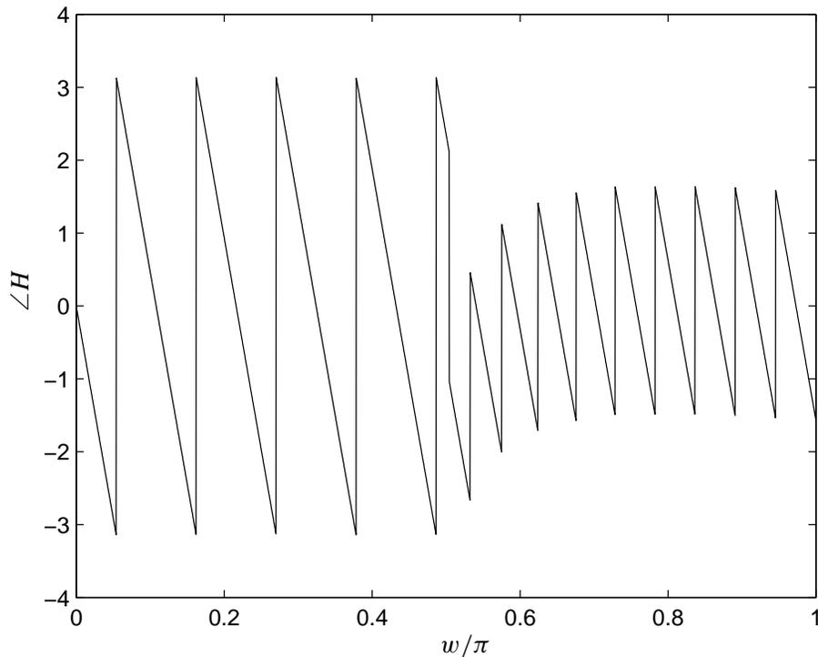
Figure 19: Phase of the frequency response of the FIR filter
