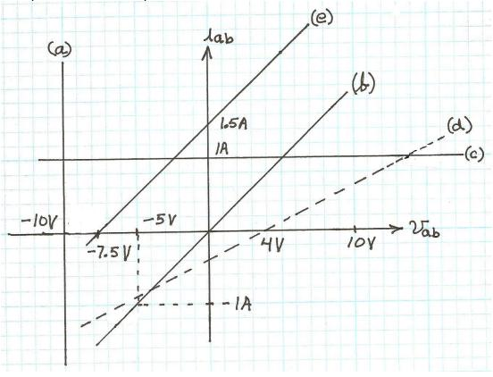
**P1.66** (a) The 1- $\Omega$  resistance, the 2- $\Omega$  resistance, and the voltage source  $\nu_x$  are in series.
