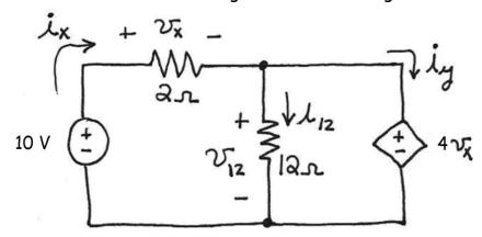
Applying KVL around the periphery of the circuit, we have  $-10 + \nu_x + 4\nu_x = 0$ , which yields  $\nu_x = 2$  V. Then, we have  $\nu_{12} = 4\nu_x = 8$  V. Using Ohm's law we obtain  $i_{12} = \nu_{12}$  /12 = 0.667 A and  $i_x = \nu_x$  /2 = 1A. Then KCL applied to the node at the top of the 12- $\Omega$  resistor gives  $i_x = i_{12} + i_y$  which yields  $i_y = 0.333$  A.
