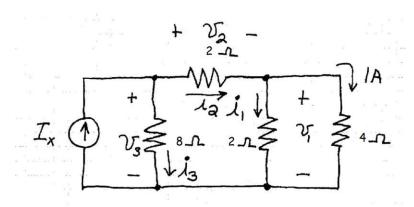
Ohm's law for the 4- $\Omega$  resistor yields:  $v_1=4$  V. Then, we have  $i_1=v_1/2=2$  A. Next, KCL yields  $i_2=i_1+1=3$  A. Then for the top 2- $\Omega$  resistor, we have  $v_2=2i_2=6$  V. Using KVL, we have  $v_3=v_1+v_2=10$  V. Next, applying Ohms law, we obtain  $i_3=v_3/8=1.25$  A. Finally applying KCL, we have  $I_x=i_2+i_3=4.25$  A.
