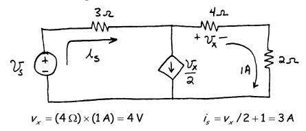
Applying KVL around the outside of the circuit, we have: (4.13 - 15)
