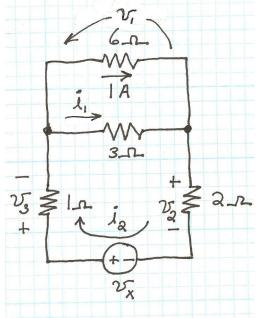
(b) The  $6-\Omega$  resistance and the  $3-\Omega$  resistance are in parallel.
