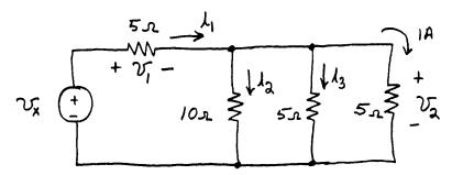
Applying Ohm's law, we have  $v_2 = (5 \Omega) \times (1 A) = 5 V$ . However,  $v_2$  is the voltage across all three resistors that are in parallel. Thus,
